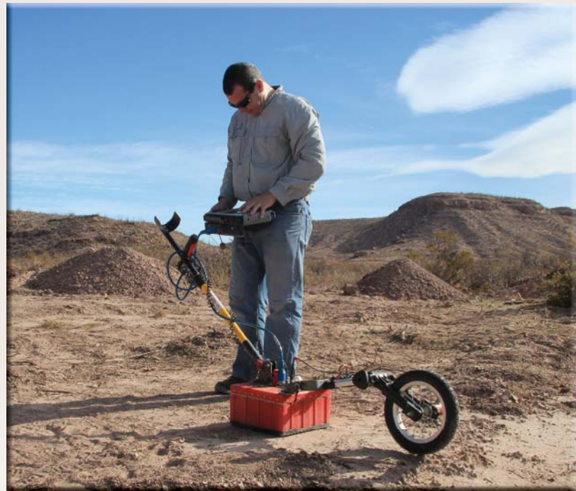
Chet Walker uses ground penetrating radar to identify subsurface anomalies.
